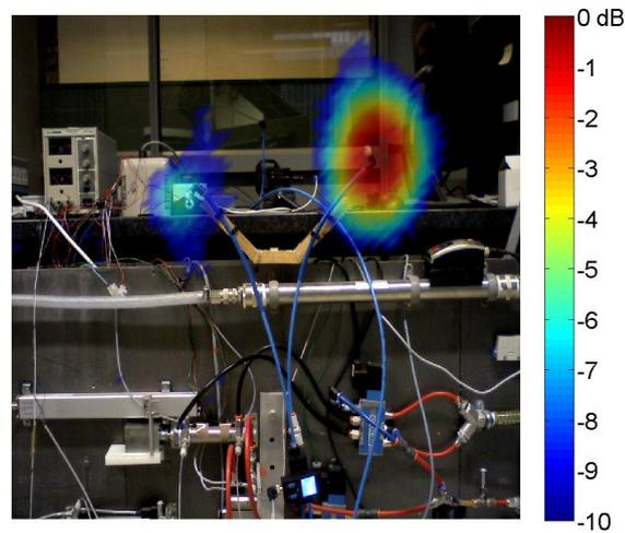
*Figure 11: Time domain beamforming with diagonal deletion (2-20kHz): two open blows at higher pressure level.*
