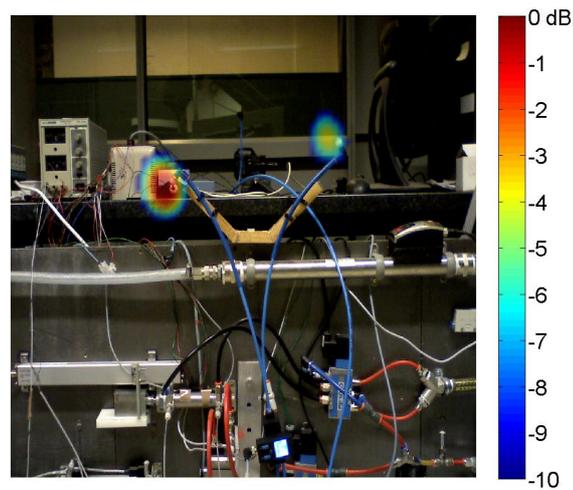
*Figure 16: Orthogonal beamforming @15.5kHz: two open blows with dominant source in the behind, second mode.*
