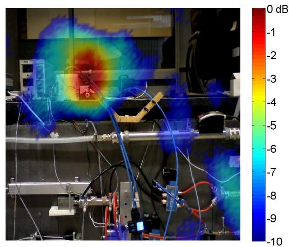
Figure 7: Time domain beamforming with diagonal deletion (2-20kHz): two close open blows at low pressure level.
