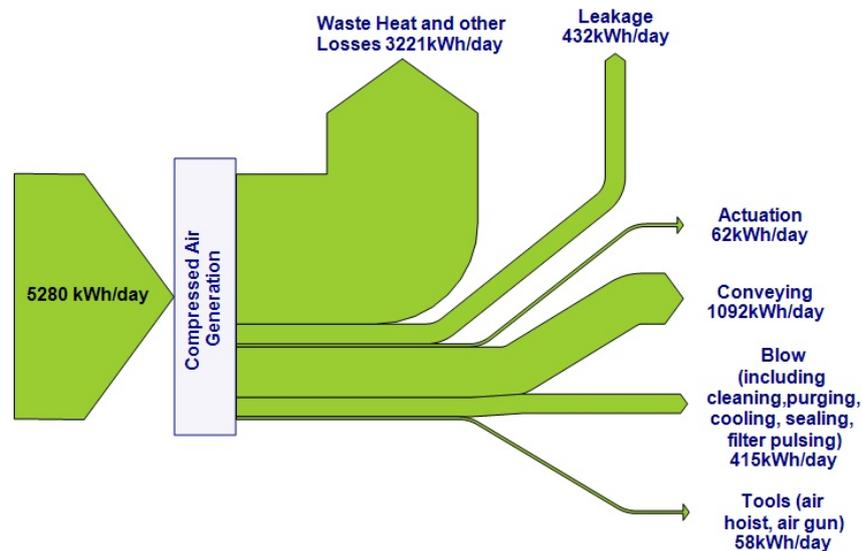
Figure 1: Example of compressed air energy flows, Eret *et al.* [4].
