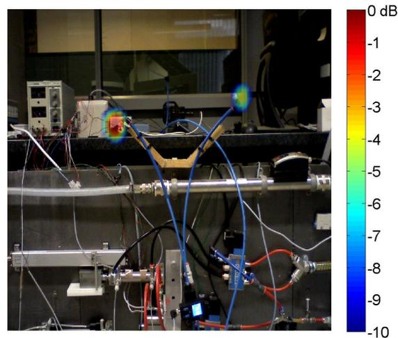
Figure 13: Frequency domain beamforming with diagonal deletion @15.5kHz: two open blows at higher pressure level.
