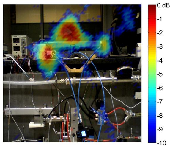
Figure 14: Time domain beamforming with diagonal deletion (2-20kHz): two open blows with dominant source in the behind.
