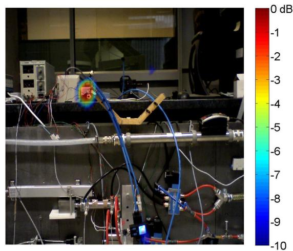
*Figure 9: Orthogonal beamforming @15.5kHz: two close open blows at low pressure level, first mode.*
