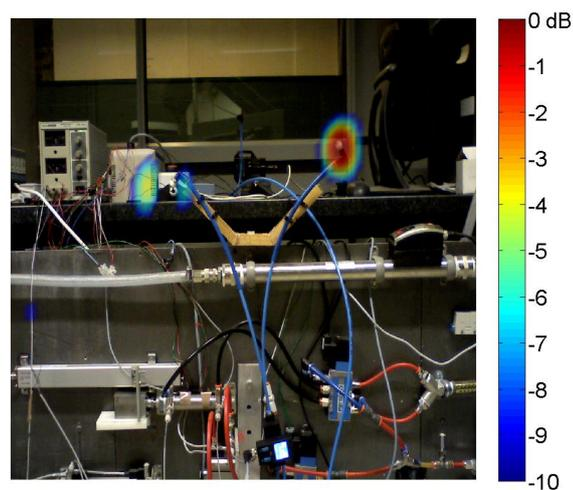
*Figure 17: Orthogonal beamforming @15.5kHz: two open blows with dominant source in the behind, third mode.*
