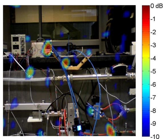
Figure 8: Frequency domain beamforming with diagonal deletion @15.5kHz: two close open blows at low pressure level.
