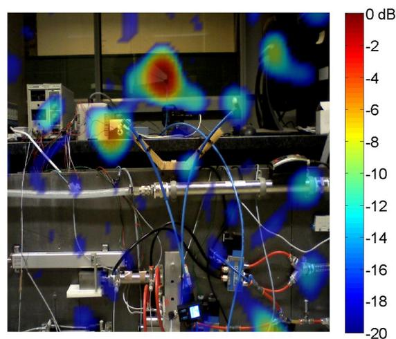
Figure 15: Frequency domain beamforming with diagonal deletion @15.5kHz: two open blows with dominant source in the behind.
