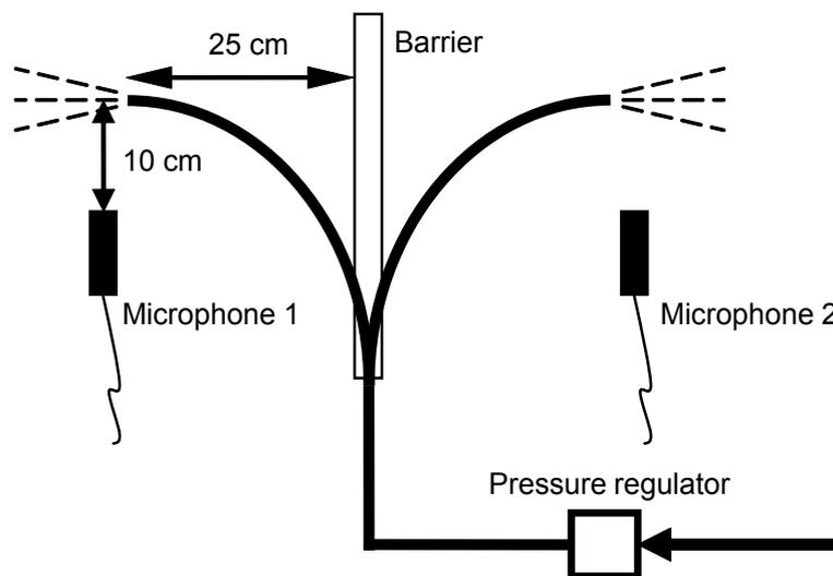
Figure 2: A schematic of two open blows test.
