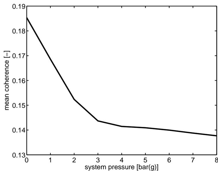
Figure 6: Mean coherence over audible frequency range at various pressure levels.
