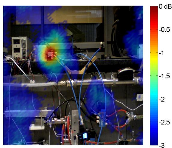
*Figure 12: Time domain beamforming (2-20kHz): after successive deletion of the main source on the right.*
