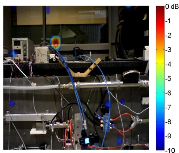
*Figure 10: Orthogonal beamforming @15.5kHz: two close open blows at low pressure level, second mode.*
