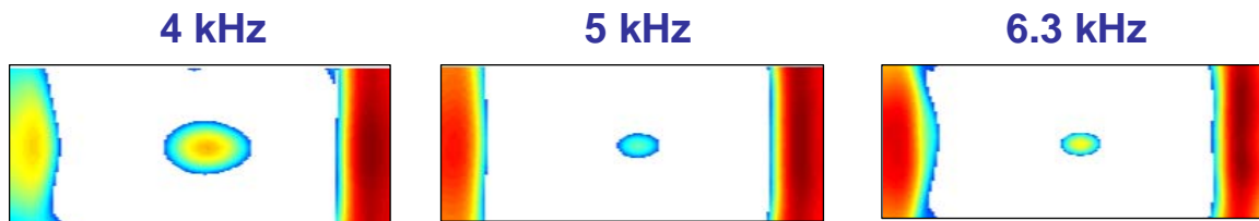
Figure 5-2-Beamforming source maps for model T0 using an adapted scanning grid (HF array)
