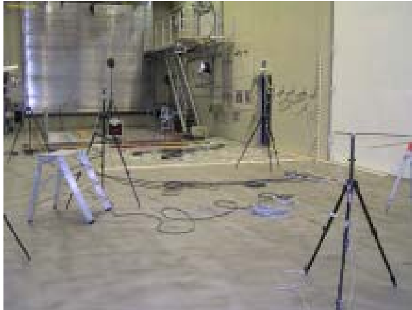
Fig. 2. The engine test cell at Rolls-Royce, Dahlewitz with the omnidirectional sound source, individual microphones and the microphone arrays
